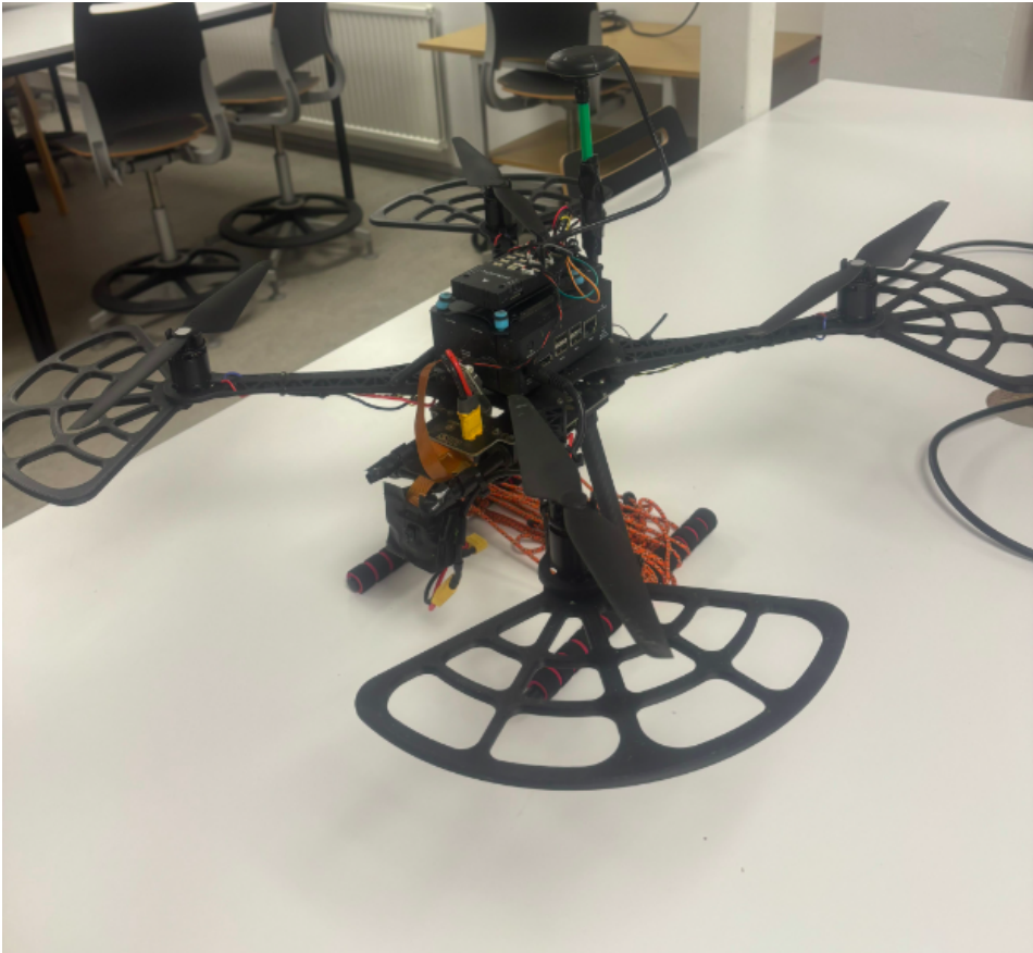
Figure 6. Physical drone, that includes the mentioned Jetson onboard computer, IMX219 camera, Pixhawk 6c flight controller
